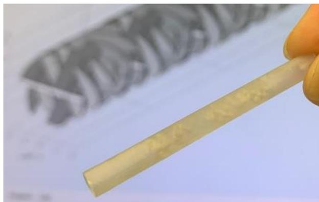
Figure 8: 3D-printed SMX mixer with 6 mixing elements A
