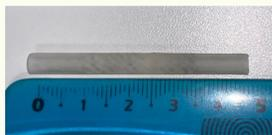
Fig. 8: 3D- printed mixer E
