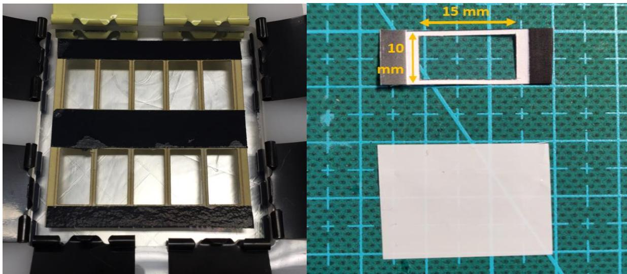
Figure 4. Sweat Sensor Manufacturing Procedures. a) Left: Applying paper frames on sensor. b) Right: A piece of membrane on paper frames and sacrificial film at the bottom
