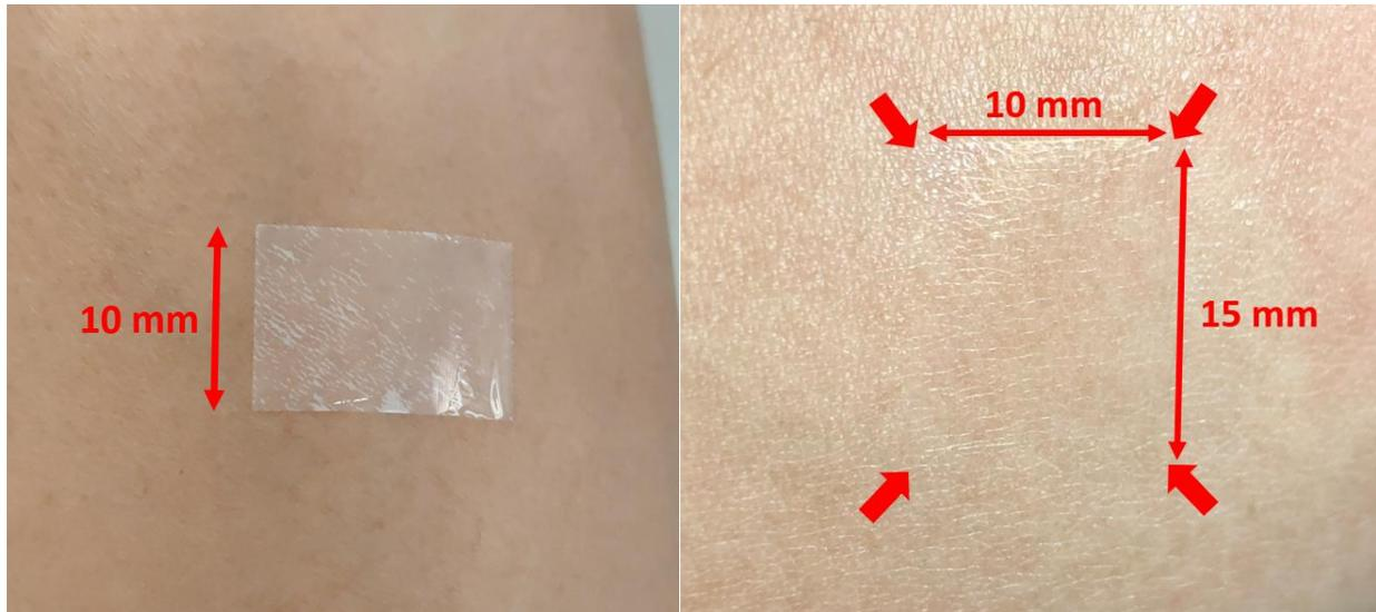
*Figure 5. Sweat sensor-P installation. a) Left: Sensor and sacrificial film. b) Right: sensors (the arrows in the figure labels the sensor corners)*
