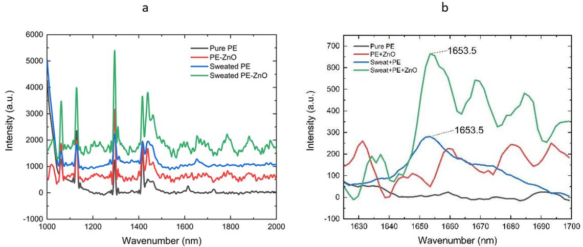
Figure 6. Raman spectrum of four samples: Pure PE (Control Sensor-P), PE + ZnO (Control Sensor-C), Sweated PE (Sample Sensor-P) and Sweated PE + ZnO (Sample Sensor-C). a) Left: 1000-2000  $\text{cm}^{-1}$  and b) Right: 1600-1700  $\text{cm}^{-1}$  that shows the presence of cortisol in Raman spectrum at 1653  $\text{cm}^{-1}$
