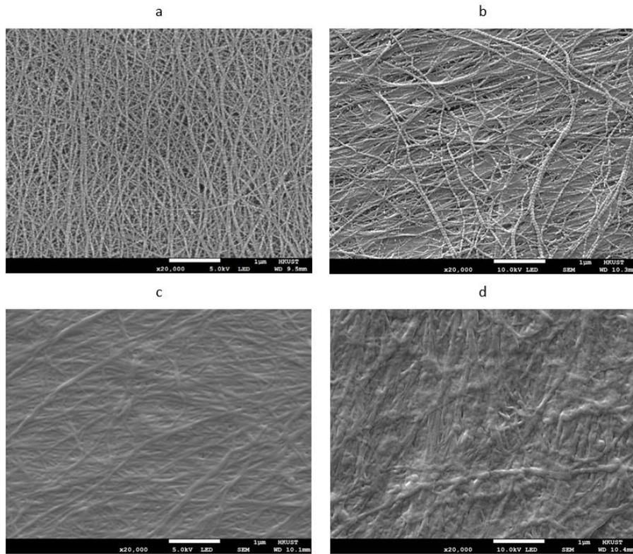
Figure 7. SEM micrographs: a) Sensor-P. b) Sensor-C. c) Sweated Sensor-P. d) Sweated Sensor-C
