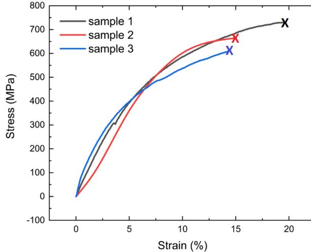
Figure 2. The complete stress vs strain curve of three different membranes ('x' marks the break point)
