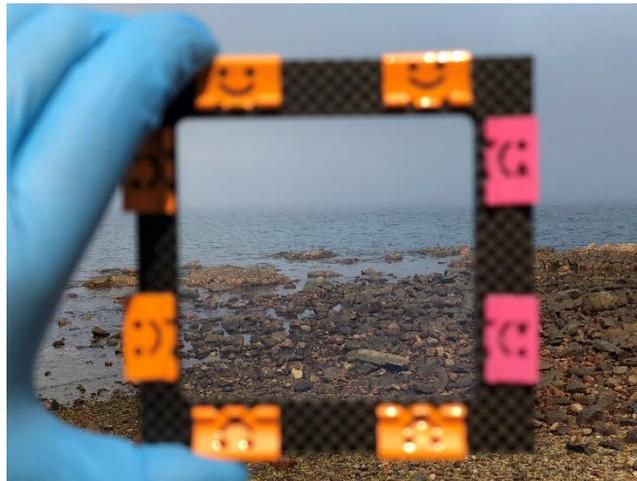
Figure 3. Nanometer Thickness Membrane held with Carbon Frames
